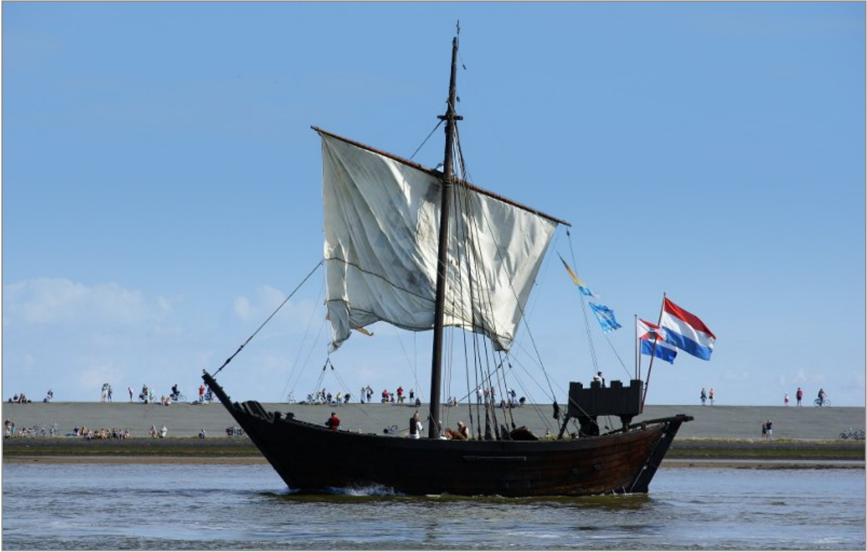
Figure 7. Reconstruction of cog, called the Kamper Hanze Kogge, from the Netherlands. This reconstruction is based on a cog-find of the fourteenth century, found in the Flevopolders
